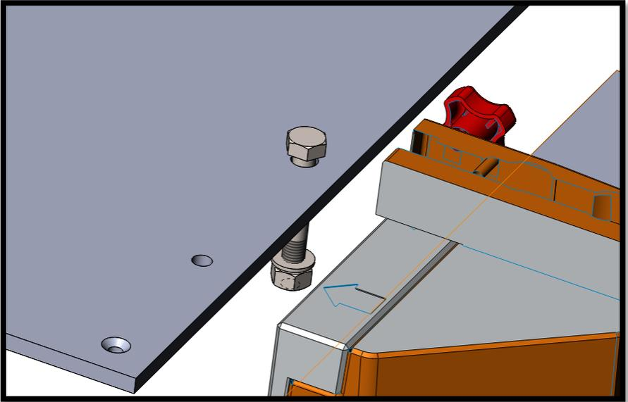
7. Slide the Fence over the M10 bolts, capturing the top of each bolt in the bottom T-slot of the fence profile. After the Fence is in place, and alignment is checked with the saw, tighten all nuts using a 16mm socket/wrench, or with a crescent wrench.
