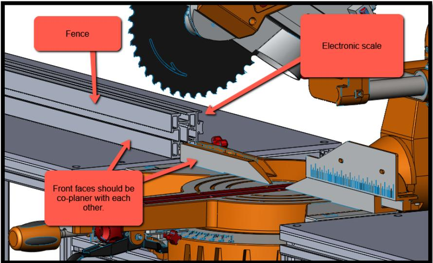
2. Align the fence so it is co-planer with any existing fences on the saw. (If there is not an existing fence, install the fence so it is perpendicular to the saw blade.
