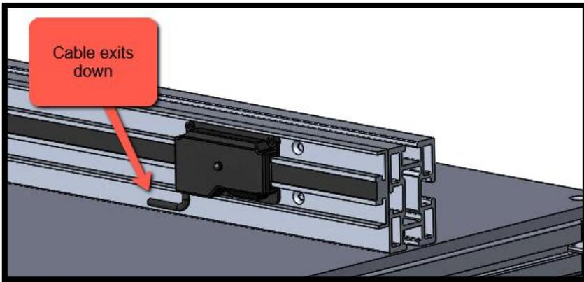
2. Attach the readout bracket to the back of the sliding stop assembly. Tighten bolts.
