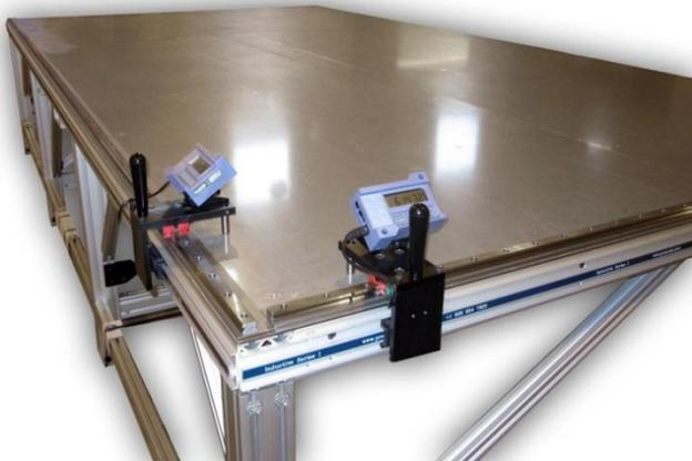
**ProTable-XY** is a two-axis measuring system designed for panel or sheet type products.
