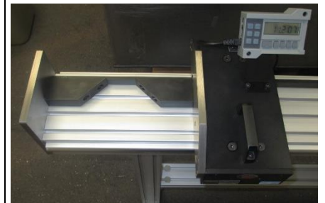
Custom inserts allow measurement of SHORT leg on mitered parts plus overall length measurement. Changeover time is less than 1 second.
