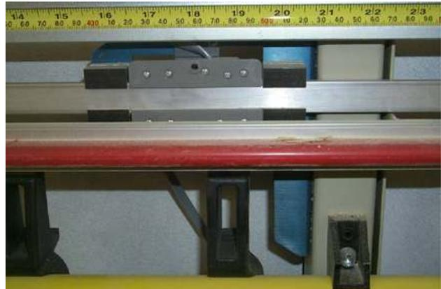
When the ProKit is properly installed, the horizontal stop moves without interference with other components.
