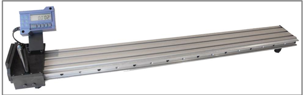
A battery powered readout travels with the moving carriage, and can perform absolute/incremental measurements, send measurements using the built-in SPC port, perform Go/NoGo testing, some statistics on parts being measured, and many more functions.
