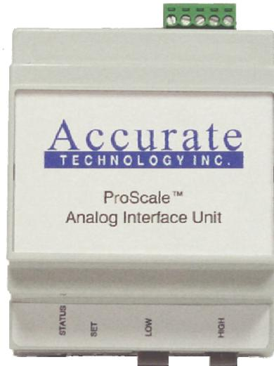
The Analog Interface Unit, or AIU, is an interface device that provides the user of a ProScale measurement system with a method of generating an analog DC output voltage that is proportional to the currently displayed ProScale position. This output can be used with an A/D converter input on a PLC or other device that utilizes an analog input signal.
