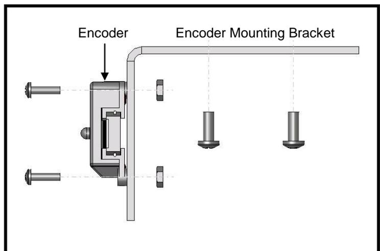
3. Mount the side of the bracket without the Encoder. Because of the wide variety of possible mounting surfaces and mounting positions, this step requires you to choose the best screws/nuts to mount the bracket.
