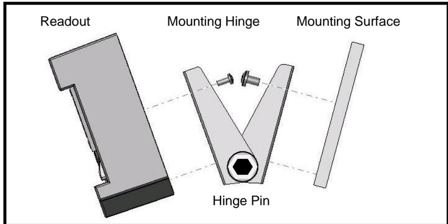
3. Use the Hinge Mounting Screws (8-32 x ¼") to mount the other side of the hinge to the mounting location determined earlier. To adjust the angle of the hinge, loosen the hinge pins with an M5 hexdriver and adjust to the desired angle. Retighten the hinge pins.
