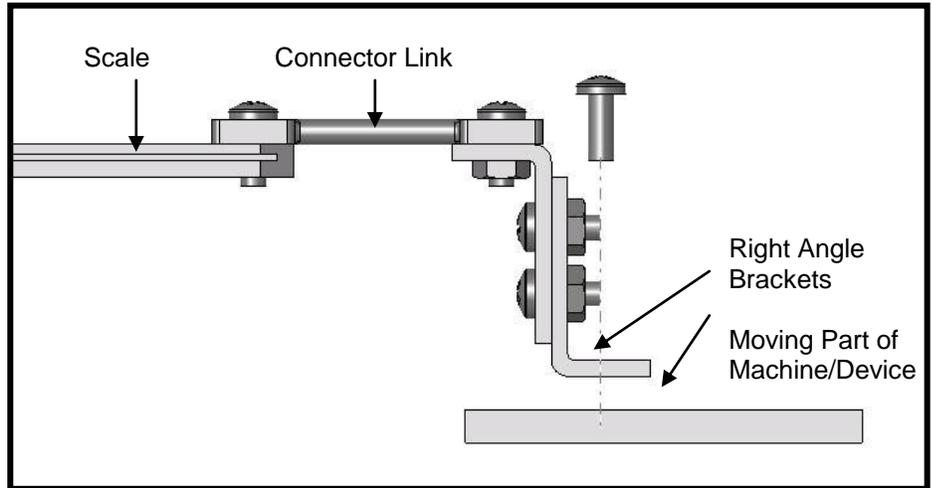
3. Attach one end of the right angle bracket assembly to the bottom of the connector link.
