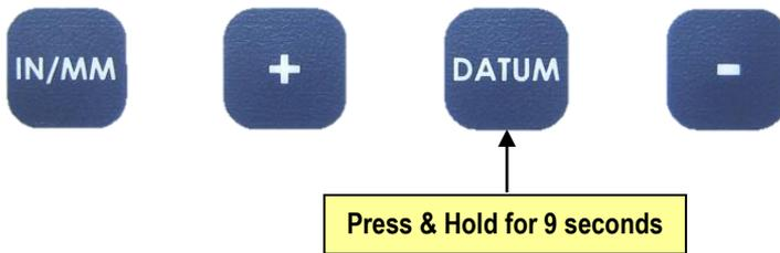
Once you are in the Programming mode, momentarily pressing the **IN/MM** key will advance through the Programming Parameter list, first displaying the Programming Parameter number, Pr x, then the currently programmed value for that parameter.
