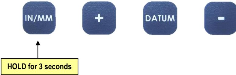
The Compact readout provides the ability to make relative, or incremental, measurements and still retain the measurements system's absolute position in memory. To enter the Incremental (or return to Absolute) measurement mode, press and hold the **IN/MM** key for 3 seconds. The **ABS** or **INC** indicator will illuminate on the display.
