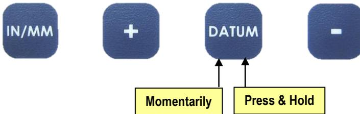
Momentarily pressing the **DATUM** key forces the readout to a user programmed value. This can value can be zero or any other [displayable value](#).
