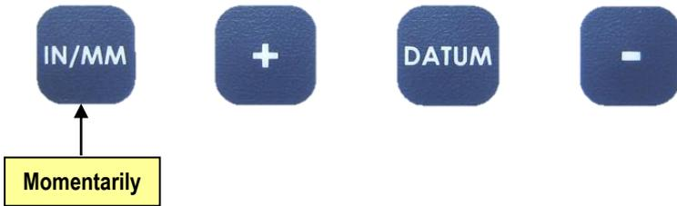
The Compact readout can display measurement/position information in inches, fractions or millimeters. To change the display mode, momentarily press the **IN/MM** key. With each key press, the DRO cycles through decimal inches, fractions (16ths, 32nds, 64ths) and millimeters.
