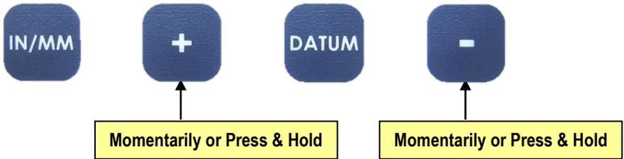
Momentarily pressing the **+** or **-** key increments or decrements the currently displayed value by one unit of measurement.
