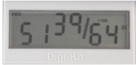
When the measurement is greater than 99 63/64 inches, a **+100** and/or **+200** will illuminate in the upper right portion of the display to indicate this amount must be added to the displayed reading. ie: If the measurement is 154 5/8 inches, 54 5/8 and **+100** will be illuminated on the display. If the measurement is -307 23/64 inches, - 7 23/64, **+100** and **+200** will be illuminated on the display.
