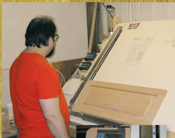
Operator checks squareness and X & Y measurements
