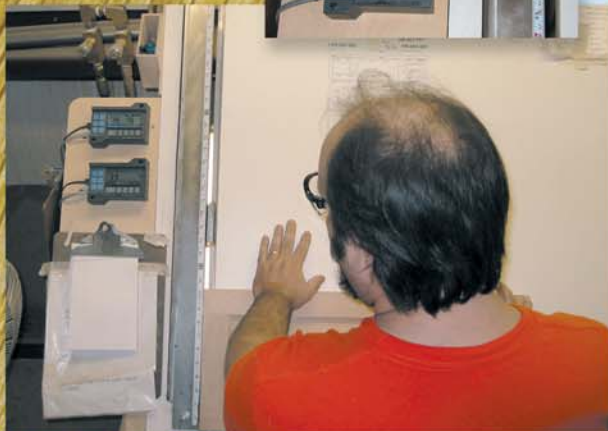
Operator checks squareness and X & Y measurements
