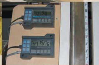
Operator checks squareness and X & Y measurements
