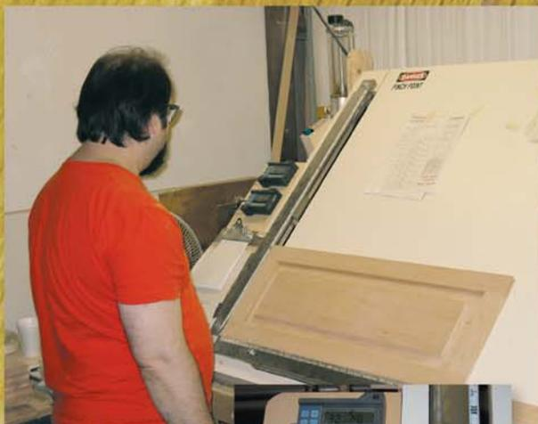
Operator checks squareness and X & Y measurements
